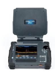
detect transmitting electronic surveillance devices and ensure that spectrum activity is captured.
